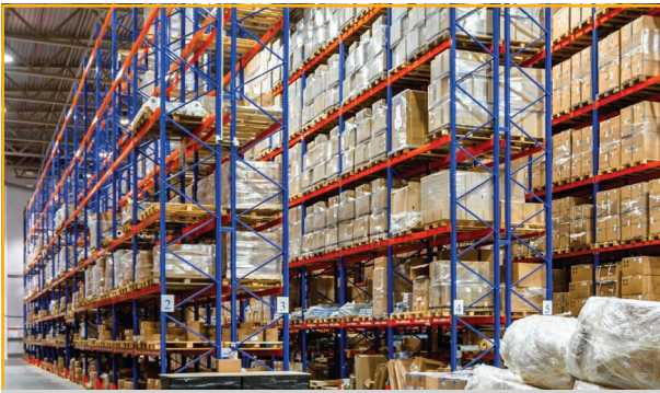
SELECTIVE PALLET RACKING
