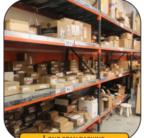
LONG SPAN RACKING
